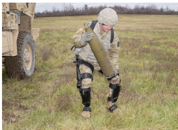
Exoskeleton makes it easier for an American soldier to lift heavy loads – here, for example, an artillery shell. Picture from an exoskeleton Operations and Maneuver and Technology Interchange meeting, 2018. [US Army]
